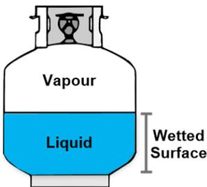
The surface area inside the cylinder which is bathed in liquid is called the 'wetted surface'. This is the area where the liquid draws heat through the cylinder walls for vaporisation.
